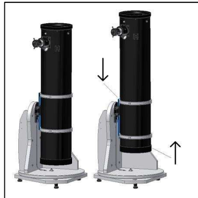
Figure B. Move the dovetail down and the tube up!
